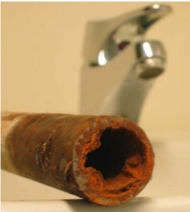
Figure 4.3: Corrosion clusters can result in poor water quality and clogging of the pipes (Photo: Eyvind Andersen)
