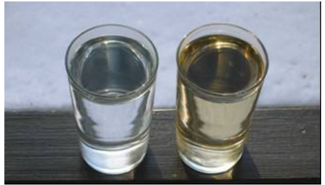
Figure 8.2: Water discoloured by humic material needs more chlorine than clear water to achieve a proper disinfection (Photo: Bjørn Løfsgaard)
