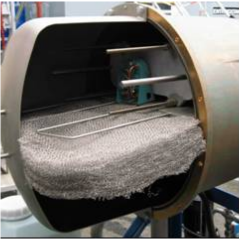
Figure 6.4: Shows the inside of an evaporator. The net prevents sea water drops from passing on to the distillate (Photo: Bjørn Løfsgaard)
