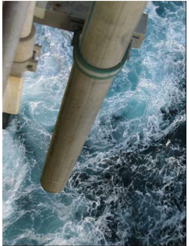
Figure 7.4: When flush valve and the bunkering hose have corresponding diameters the system can be flushed with maximum pressure. (Photo: Eyvind Andersen)
