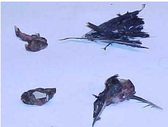
Figure 9.1: Pieces of a dead bird found in a potable water tank. The bird entered via the bunkering pipe, was caught in a valve and spread to all water storage tanks as the body decomposed (Photo: The picture is used anonymously in agreement with the company)
